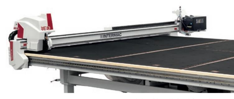
The base of the machine is made from a rigid, rectangular structure onto which ground wood panels are attached, ensuring maximum planarity of the working area, essential for optimal glass grooving and break-out operations.
