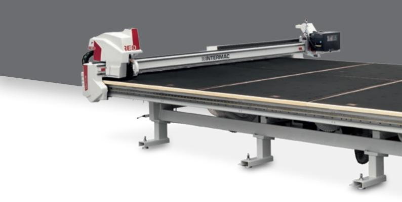
**Genius CT-RED** is the range of high-performance cutting tables for both **REGULAR** and **JUMBO** sheets of float glass, for working on cutting lines over two or three shifts. It provides maximum productivity, reliability and durability over time, courtesy of quality components and cutting-edge technological solutions that guarantee continuous cycle, maintenance-free machining precision.
