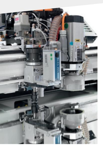
Genius CT-RED can perform low emissivity (Low-E) removal operations, thanks to a series of optional devices dedicated to the various production requirements.
